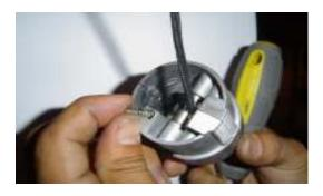
10) IF PIN IS MISSING AND LOOSE INSIDE CRANK ASSEMBLY, CRANK ASSEMBLY NEEDS TO BE REPLACED. (SOMETHING IS WRONG IF PIN IS NOT HOLDING IN PLACE.)
