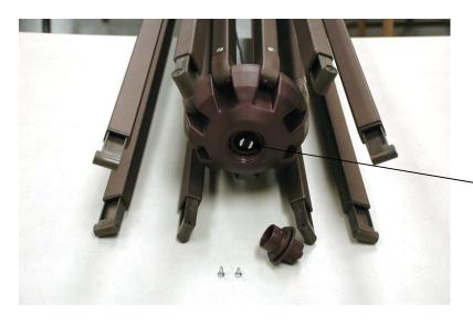
**D.** Push sleeve back into lower hub to expose cord lock assembly.
