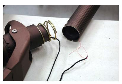
11. Re-attach string with strong knot, carefully pull umbrella cord thru Arm Pole; Top Notch; and Lower Hub.
