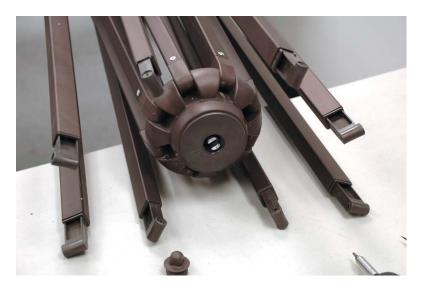
15. If step #13 & #14 are properly done, cord lock should be just inside of lower hub (as illustrated on photo).
