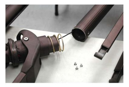
**6.** Separate Arm Pole from Tilt Assembly by gently pulling it apart.
