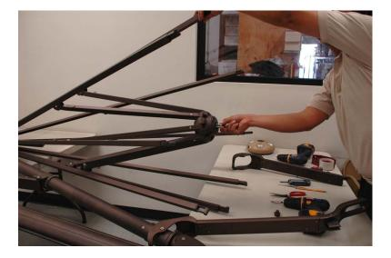
**14.** While opening the canopy frame with hand, rotate (tighten) the cord lock another 1/2 turn and insert into cavity at lower hub.
