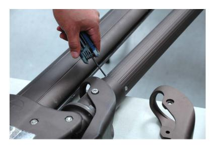
**5.** Remove 3 screws located near bottom of Arm Pole, safe keeping screws for re-Assembly use.
