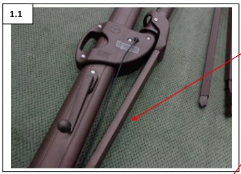
Remove the AKZ from the rotating hub by unscrewing the main frame bolts at the bottom of the main frame stand.
