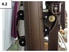
Remove the nuts and half of the main frame grip.
