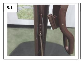
Using the hex wrench, remove the bolt holding the loop lock stopper in place.
