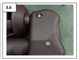
Replace other half of hinge and tighten bolts to hold it in place. Then replace cotter pin.
