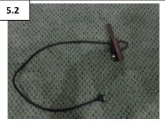
Pull cord through the center of the loop lock stopper to create a small loop. Then remove it from the frame.
